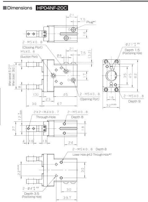
\*1) Two faces have an air port. Select the one you use according to the mounting condition.
