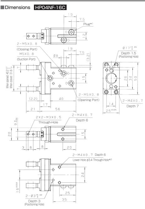
\*1) Two faces have an air port. Select the one you use according to the mounting condition.
